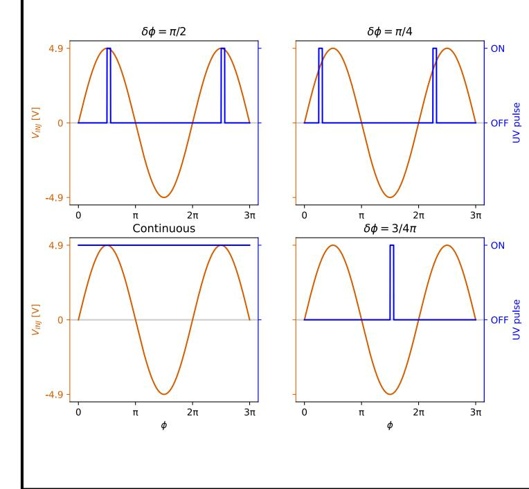
Injection Electrodes ±4.9 V at ~98Khz sine
