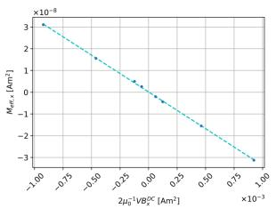
Δg acceleration demodulated at the injected frequency against the gradient of the AC field have  $M_{eff,x}$  as the slope of the fit.  $M_{eff,x}$ linear dependence with the DC field determines  $M_{r}$  as the offset and  $\chi$  as the slope
