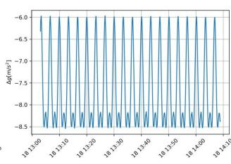
Δg acceleration demodulated at twice the injected frequency provides results of the magnetic susceptibility
