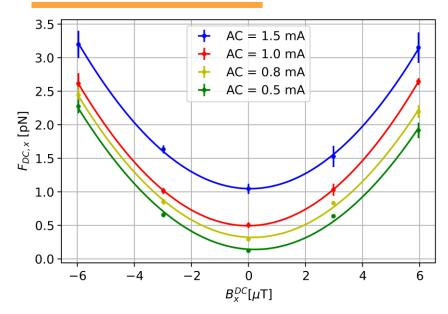
A quadratic fit of the dependence of  $F_{DC,x}$  with the injected DC field allows the determination of  $\chi_{DC}$ ,  $B_{back,x}$  and  $\nabla_x B_{back,x}$ .
