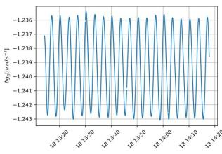
Δg rotations demodulated at the injected frequency allow determination of  $M_{\nu}$  and  $M_{z}$
