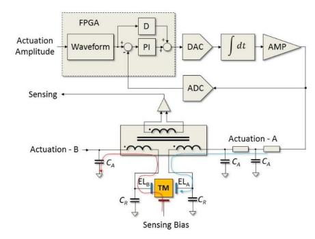
$$F_q(t) = rac{1}{2} \left| rac{\partial C_q^*}{\partial q} \right| \left( V_{m_1}^2(t) + V_{m_2}^2(t) - V_{m_3}^2(t) - V_{m_4}^2(t) \right)$$
