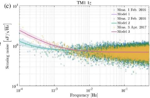
$$\left(1 \frac{aF}{\sqrt{Hz}}\right)^2 \left[1 + \left(\frac{1 \, mHz}{f}\right)\right] + \left(\Delta C \, 30 \times 10^{-6} \, \frac{aF}{\sqrt{Hz}}\right)^2 \left(\frac{1 \, mHz}{f}\right)$$
