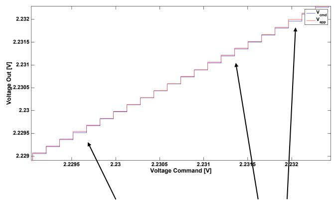
Differences between the commanded and applied voltages Fully deterministic i.e. Predictable and repeatable
